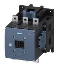
power contactor, AC-3e/AC-3 400 A, 200 kW / 400 V AC (50-60 Hz) / DC Uc: 96-127 V PLC input 24 V DC 3-pole, auxiliary contacts 2 NO + 2 NC drive: electronic main circuit: busbar control and auxiliary circuit: screw terminal
