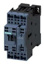
power contactor, AC-3e/AC-3, 32 A, 15 kW / 400 V, 3-pole, 125 V DC, auxiliary contacts: 1 NO + 1 NC, spring-loaded terminal, size: S0  $\,$
