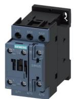
power contactor, AC-3e/AC-3, 38 A, 18.5 kW / 400 V, 3-pole, 400 V AC, 50 Hz / 400-440 V, 60 Hz, auxiliary contacts: 1 NO + 1 NC, screw terminal, size: S0
