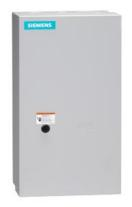
Mechanically held lighting contactor, Contactor amp rating 200A, 0 N.C. / 2 N.O. poles, 110VAC 50HZ/120VAC 60HZ coil, Non-combination type, Enclosure NEMA type 1, Indoor general purpose use
