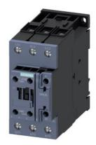
power contactor, AC-3e/AC-3, 80 A, 37 kW / 400 V, 3-pole, 20-33 V AC/DC, 50/60 Hz, with integrated varistor, auxiliary contacts: 1 NO + 1 NC, screw terminal, size: S2
