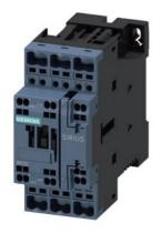
power contactor, AC-3, 25 A, 11 kW / 400 V, 4-pole, 220 V DC, main contacts: 2 NO + 2 NC, auxiliary contacts: 1 NO + 1 NC, spring-loaded terminal, size: S0
