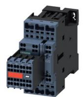
power contactor, AC-3e/AC-3, 25 A, 11 kW / 400 V, 3-pole, 24 V DC, with pluggedin varistor, auxiliary contacts: 2 NO + 2 NC, spring-loaded terminal, size: S0, captive auxiliary switch
