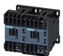
reversing contactor assembly, AC-3e/AC-3, 7 A, 3 kW / 400 V, 3-pole, 48 V AC, 50/60 Hz, spring-loaded terminal, electrical and mechanical interlock
