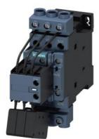
capacitor contactor, AC-6b 33 kVAr, / 400 V, 3-pole, 110 V DC, auxiliary contacts: 1 NO + 2 NC, screw terminal, size: S0
