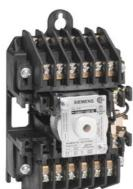
Mechanically held lighting contactor, Contactor amp rating 20A, 0 N.C. / 10 N.O. poles, Non-combination type, Enclosure NEMA type (open), No enclosure  $% 10^{-1}$
