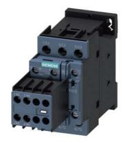
power contactor, AC-3e/AC-3, 38 A, 18.5 kW / 400 V, 3-pole, 110 V AC, 50 Hz, auxiliary contacts: 2 NO + 2 NC, screw terminal, size: S0, removable auxiliary switch
