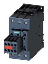
power contactor, AC-3e/AC-3, 80 A, 37 kW / 400 V, 3-pole, 110 V AC, 50 Hz / 120 V, 60 Hz, with plugged-in varistor, auxiliary contacts: 2 NO + 2 NC, screw terminal, size: S2, captive auxiliary switch
