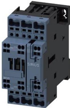
power contactor, AC-3e/AC-3, 25 A, 11 kW / 400 V, 3-pole, 110 V AC, 50 Hz / 120 V, 60 Hz, auxiliary contacts: 1 NO + 1 NC, spring-loaded terminal, size: S0, multi-unit packaging, pack = 18 units
