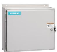
Mechanically held lighting contactor, Contactor amp rating 30Amp 0NC \_ 6NO poles, 440VAC 50HZ/480VAC 60HZ coil, Non-combination type, Enclosure NEMA type 12, Dust/drip proof for indoors
