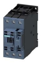
traction contactor, AC-3e/AC-3, 51 A, 22 kW / 400 V, 3-pole, 24 V DC, 0.7-1.25\* Us, electronic drive, with integrated varistor, auxiliary contacts: 1 NO + 1 NC, main circuit: screw terminal, control and auxiliary circuit: spring-loaded terminal, size: S2
