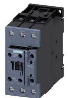
power contactor, AC-3e/AC-3, 41 A, 18.5 kW / 400 V, 3-pole, 400 V AC, 50 Hz / 400-440 V, 60 Hz, auxiliary contacts: 1 NO + 1 NC, screw terminal, size: S2
