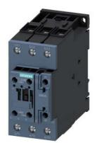
power contactor, AC-3e/AC-3, 41 A, 18.5 kW / 400 V, 3-pole, 20-33 V AC/DC, 50/60 Hz, with integrated varistor, auxiliary contacts: 1 NO + 1 NC, screw terminal, size: S2, communication-capable
