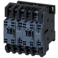
reversing contactor assembly, AC-3e/AC-3, 25 A, 11 kW / 400 V, 3-pole, 110 V AC, 50/60 Hz, spring-loaded terminal, electrical and mechanical interlock, auxiliary contacts:  $2 \times 1 \text{ NO}$
