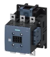
power contactor, AC-3e/AC-3 265 A, 132 kW / 400 V AC (50-60 Hz) / DC Uc: 575-600 V 3-pole, auxiliary contacts 2 NO + 2 NC drive: conventional main circuit: busbar control and auxiliary circuit: spring-loaded terminal
