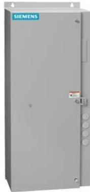
Mechanically held lighting contactor, Contactor amp rating 400A, 0 N.C. / 3 N.O. poles, 440VAC 50HZ/480VAC 60HZ coil, Non-combination type, Enclosure NEMA type 1, Indoor general purpose use
