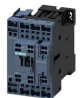
contactor AC-1, 40 A, 400 V / 40  $^\circ$ C, 4-pole, 110 V DC, auxiliary contacts: 1 NO + 1 NC, spring-loaded terminal, size: S0
