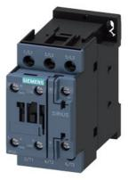
contactor, NEMA version, 10 hp, 460 / 575 V, 3-pole, 208 V AC, 50/60 Hz, auxiliary contacts: 1 NO + 1 NC, screw terminal, size: S0  $\,$
