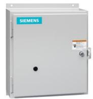
Mechanically held lighting contactor, Contactor amp rating 100A, 0 N.C. / 2 N.O. poles, 110VAC 50HZ/120VAC 60HZ coil, Non-combination type, Enclosure NEMA type 12, Dust/drip proof for indoors
