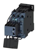
capacitor contactor, AC-6b 25 kVAr, / 400 V, 3-pole, 200-280 V AC/DC, 50/60 Hz, with integrated varistor, auxiliary contacts: 1 NO + 2 NC, screw terminal, size: S0  $\,$
