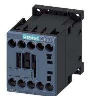
power contactor, AC-3e/AC-3, 16 A, 7.5 kW / 400 V, 3-pole, 60 V DC, auxiliary contacts: 1 NO, screw terminal, size: S00  $\,$
