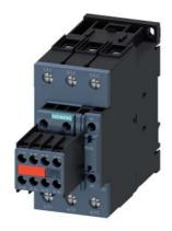
power contactor, AC-3e/AC-3, 80 A, 37 kW / 400 V, 3-pole, 230 V AC, 50/60 Hz, with plugged-in varistor, auxiliary contacts: 2 NO + 2 NC, screw terminal, size: S2, captive auxiliary switch
