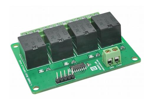
4 Channel Relay Controller Board
