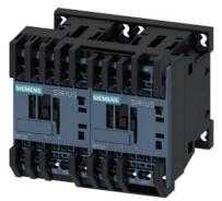
reversing contactor assembly, AC-3e/AC-3, 12 A, 5.5 kW / 400 V, 3-pole, 24 V DC, spring-loaded terminal, electrical and mechanical interlock
