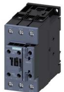
power contactor, AC-3e/AC-3, 41 A, 18.5 kW / 400 V, 3-pole, 200 V AC, 50 Hz / 200-220 V, 60 Hz, auxiliary contacts: 1 NO + 1 NC, screw terminal, size: S2
