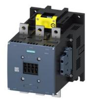
power contactor, AC-3e/AC-3 400 A, 200 kW / 400 V AC (50-60 Hz) / DC 200-277 V x (0.8-1.1) F-PLC input 24 V DC 3-pole, auxiliary contacts 2 NO + 2 NC drive: electronic main circuit: busbar control and auxiliary circuit: screw terminal
