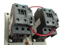
Electrically held lighting contactor, Contactor amp rating 30A, 0 N.C. / 6 N.O. Poles, 277VAC 60HZ coil, Non-combination type, (no disconnect device), Enclosure NEMA type (open), No enclosure
