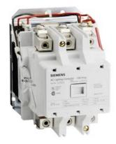
Mechanically held lighting contactor, Contactor amp rating 100A, 0 N.C. / 3 N.O. poles, 208VAC 60HZ coil, Non-combination type, Enclosure NEMA type (open), No enclosure
