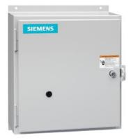
Mechanically held lighting contactor, Contactor amp rating 30A, 0 N.C. / 12 N.O. poles, 440VAC 50HZ/480VAC 60HZ coil, Non-combination type, Enclosure NEMA type 1, Indoor general purpose use
