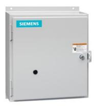
Mechanically held lighting contactor, Contactor amp rating 30A, 0 N.C. / 12 N.O. poles, 277VAC 60HZ coil, Non-combination type, Enclosure NEMA type 1, Indoor general purpose use
