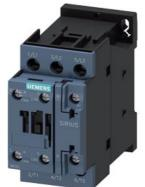
power contactor, AC-3e/AC-3, 38 A, 18.5 kW / 400 V, 3-pole, 230 V AC, 50 Hz, auxiliary contacts: 1 NO + 1 NC, screw terminal, size: S0
