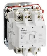
Mechanically held lighting contactor, Contactor amp rating 200A, 0 N.C. / 3 N.O. poles, 220VAC 50HZ/240VAC 60HZ coil, Non-combination type, Enclosure NEMA type (open), No enclosure
