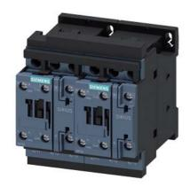
reversing contactor assembly, AC-3e/AC-3, 12 A, 5.5 kW / 400 V, 3-pole, 110 V AC, 50/60 Hz, screw terminal, electrical and mechanical interlock, auxiliary contacts: 2 x 1 NO
