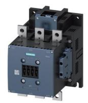
power contactor, AC-3e/AC-3 265 A, 132 kW / 400 V AC (50-60 Hz) / DC Uc: 21-27.3 V PLC input 24 V DC 3-pole, auxiliary contacts 2 NO + 2 NC drive: electronic main circuit: busbar control and auxiliary circuit: screw terminal
