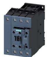
power contactor, AC-3, 40 A, 18.5 kW / 400 V, 4-pole, 230 V AC, 50/60 Hz, main contacts: 2 NO + 2 NC, auxiliary contacts: 1 NO + 1 NC, screw terminal, size: S2
