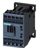
power contactor, AC-3e/AC-3, 9 A, 4 kW / 400 V, 3-pole, 24 V DC, with integrated diode, auxiliary contacts: 1 NC, spring-loaded terminal, size: S00
