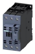
power contactor, AC-3e/AC-3, 51 A, 22 kW / 400 V, 3-pole, 20-33 V AC/DC, 50/60 Hz, with integrated varistor, auxiliary contacts: 1 NO + 1 NC, main circuit: screw terminal, control and auxiliary circuit: spring-loaded terminal, size: S2,
