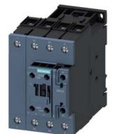
power contactor, AC-3, 51 A, 22 kW / 400 V, 4-pole, 24 V AC, 50/60 Hz, main contacts: 2 NO + 2 NC, auxiliary contacts: 1 NO + 1 NC, screw terminal, size: S2
