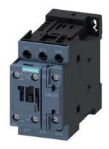
power contactor, AC-3e/AC-3, 25 A, 11 kW / 400 V, 3-pole, 200-280 V AC/DC, 50/60 Hz, with integrated varistor, auxiliary contacts: 1 NO + 1 NC, screw terminal, size: S0
