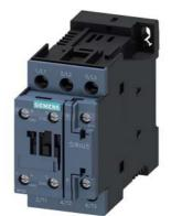
power contactor, AC-3e/AC-3, 9 A, 4 kW / 400 V, 3-pole, 95-130 V AC/DC, 50/60 Hz, with integrated varistor, auxiliary contacts: 1 NO + 1 NC, screw terminal, size: S0
