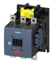
power contactor, AC-3e/AC-3 300 A, 160 kW / 400 V, AC (50-60 Hz) / DC 96-127 V x (0.8-1.1) F-PLC input 24 V DC 3-pole, auxiliary contacts 2 NO + 2 NC permanently mounted drive: electronic main circuit: busbar control and auxiliary circuit: screw terminal
