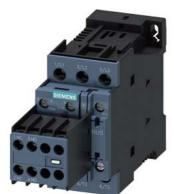
power contactor, AC-3e/AC-3, 25 A, 11 kW / 400 V, 3-pole, 110 V DC, auxiliary contacts: 2 NO + 2 NC, screw terminal, size: S0, removable auxiliary switch
