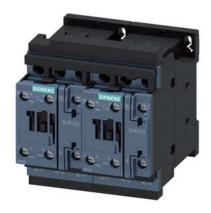
reversing contactor assembly, AC-3e/AC-3, 12 A, 5.5 kW / 400 V, 3-pole, 110 V AC, 50 Hz / 120 V, 60 Hz, screw terminal, electrical and mechanical interlock, auxiliary contacts: 2 x 1 NO
