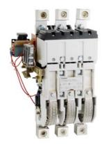
Mechanically held lighting contactor, Contactor amp rating 300A, 0 N.C. / 2 N.O. poles, 440VAC 50HZ/480VAC 60HZ coil, Non-combination type, Enclosure NEMA type (open), No enclosure
