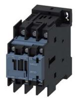
power contactor, AC-3e/AC-3, 25 A, 11 kW / 400 V, 3-pole, 24 V DC, 0.7-1.25\* Us, with integrated diode combination, auxiliary contacts: 1 NO + 1 NC, ring cable lug connection, size: S0
