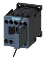
Contactor relay railway, 2 NO + 1 NC 125 V DC, 0.7 ... 1.25\* US, with integrated suppressor diode, Size S00, screw terminal installation on standard mounting rail optimized (20 G) suitable for PLC outputs
